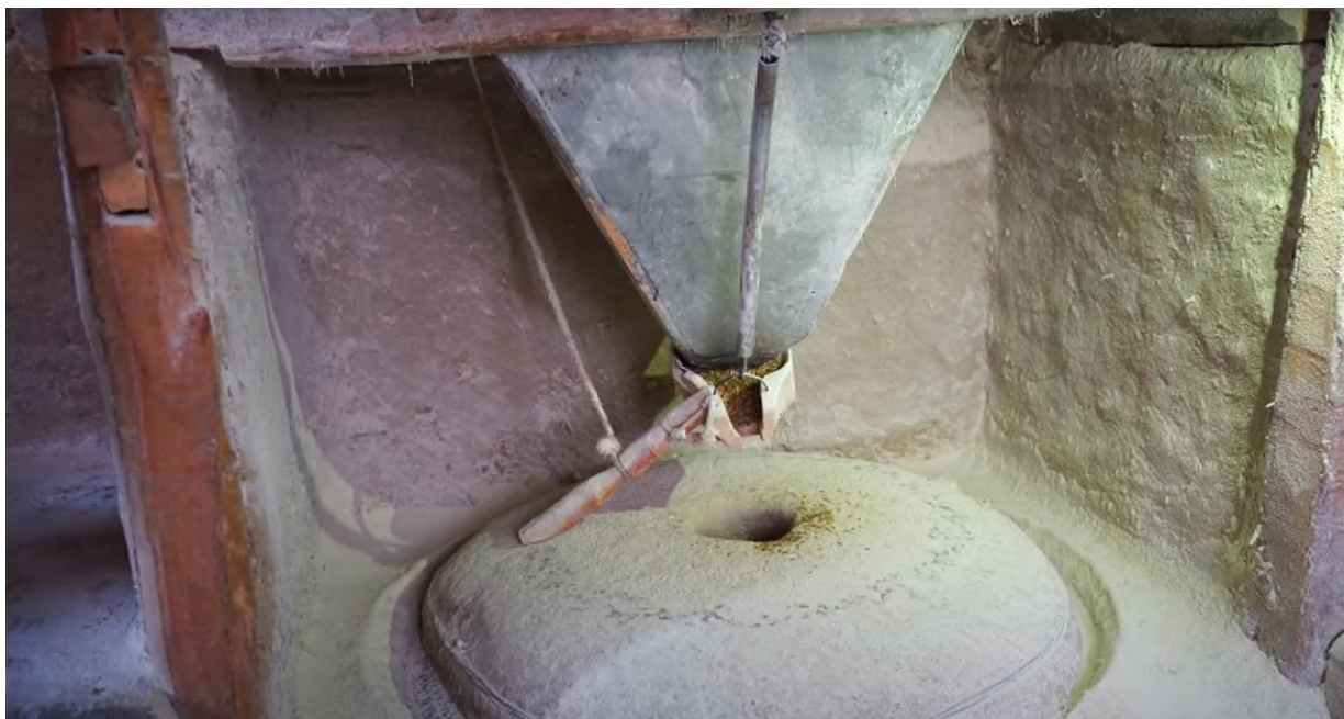
Figure 4. A stone mill powered by water for 100 years. Gelon village
